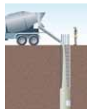
Concrete poured to form the pile.
