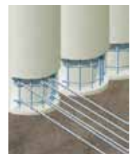
Connection of basement slab reinforcement.
